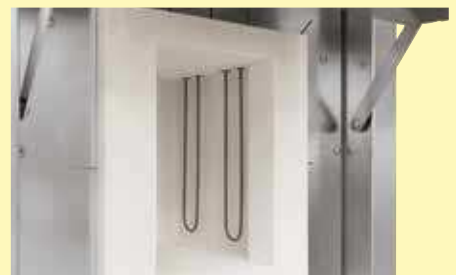
High-quality molybdenum disilicide heating elements
