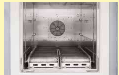
Roller conveyor in furnace chamber
