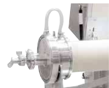
Water-cooled vacuum flange (gas supply system 2)
