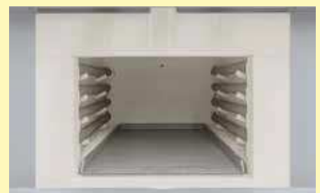
Deep furnace chamber with three-sides heating
