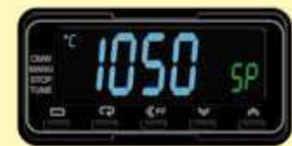
Example of an over-temperature limiter
