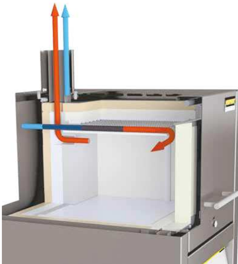
Air inlet and exhaust flow principle in ashing furnaces
