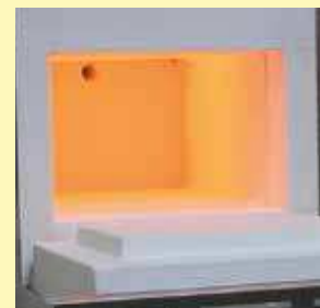
Muffle heated from four sides
