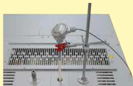
Thermocouple port in the ceiling with tripod
